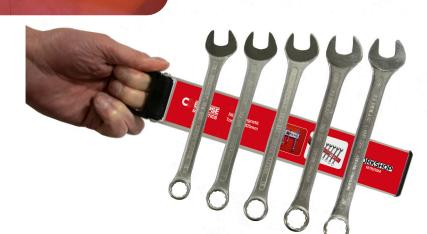
The Mobile Magnetic Tool Rack has two magnetic faces. The reverse side (darker) is the side for magnetic clamping against a ferrous surface (such as a mild steel cabinet) there is no need to use mechanical fixings such as screws. The front face is also magnetic allowing the user to place ferrous objects such as mild steel tools onto it. Ferrous tools such as spanners, screwdrivers, allan keys, etc can all be held in place.
