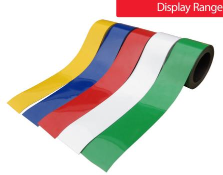
The Racking Strip & Bay Markers magnetic tapes use 0.5mm thick magnetic rubber rated at up to 28g/cm² (0.398lb/in²) of area and have a dry-wipe finish vinyl top layer (approximately 0.1mm thick). The magnetic rubber layer is magnetised multiple pole on the visible magnetic face and is slit from larger width rolls.
